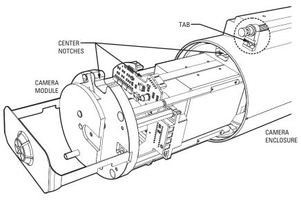
Figure 15. Install Camera Module
